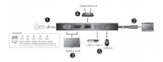
1. Plug in the power adapter to the USB-C DC in Port on your UH3236.
