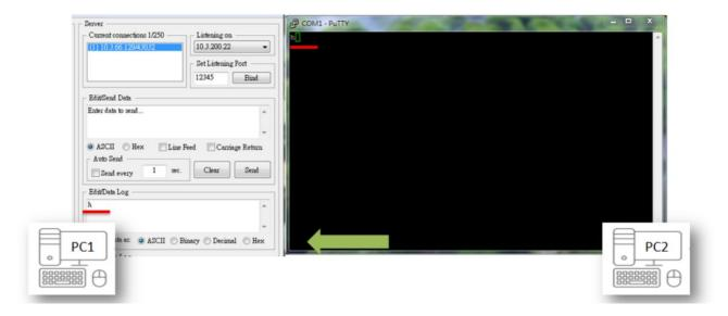
**Note**: Conversely, you can also enter any text on the TCP Test Tool of PC1 to test if it can be received by the Putty of PC2.
