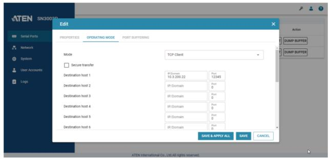
8. Optionally enable the Secure transfer option if you want the data to be encrypted and transmitted securely over a network.
