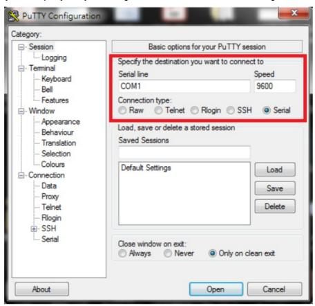
3. On the Putty of PC2 (serial device), you can enter any text to test if it can be received by the TCP Test Tool of PC1 (host), as exemplified below.
