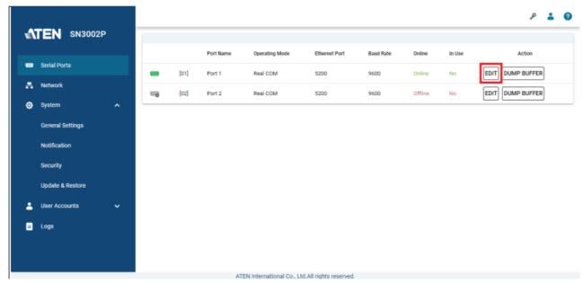
6. Under PROPERTIES, configure the necessary serial communication settings (e.g. baud rate, parity, etc.) to match with the connected serial device.
