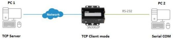
• On PC1, use TCP Test Tool, a third-party utility, to send or receive data to or from PC2, as illustrated below.
