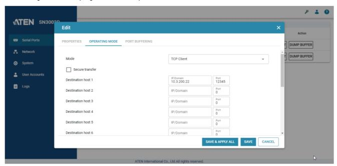
• Optionally enable the Secure transfer option if you want the data to be encrypted and transmitted securely over a network.
