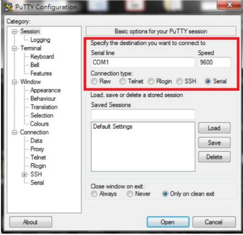
• On the Putty of PC2 (serial device), you can enter any text to test if it can be received by the TCP Test Tool of PC1 (host), as exemplified below.
