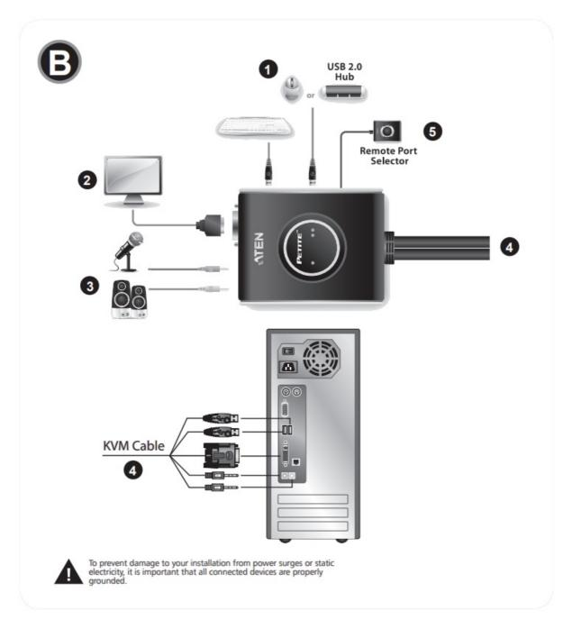
Make sure that the power to any device that you connect to the installation has been turned off. You must unplug the power cords of any computers that have the Keyboard Power On function.
