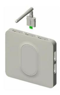
Pole Zigbee Module is suitable for Gen2 Gateway. 3 Slots of Gen2 Gateway can be used for Zigbee. To fulfill the ESL System, at least 3 Pole Zigbee Modules should be inserted to the Gateway. Likewise, this picture, when you insert modules, be careful with the directions. Modules will not be able to be put in when the inserting direction is opposite.
