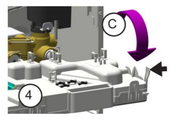
5. Remove all connectors from the top and the back side of the control uni;
