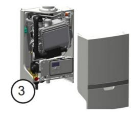
4. Push the lip C to the left and turn the control unit forward;
