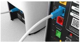
**Tip:** Make sure the Ethernet cable is firmly connected. Once both ends are properly connected, the Ethernet port LED will turn SOLID GREEN. After the extender has been paired and the front LED is SOLID WHITE, you can connect another device by Ethernet.
