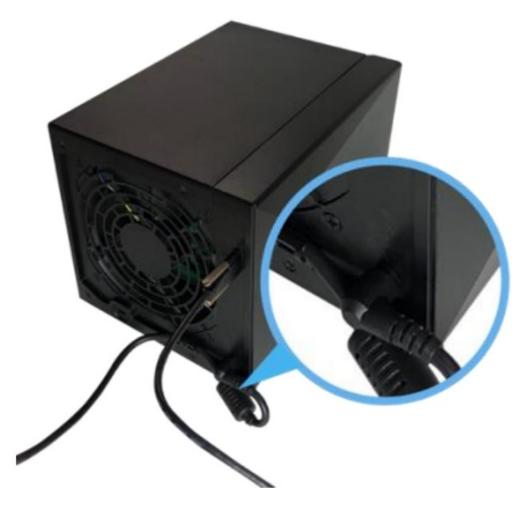
3. Connect the other end of the USB 3.2 Gen2 cable to a USB 3.2 port on your NAS, which should not be powered on yet.
