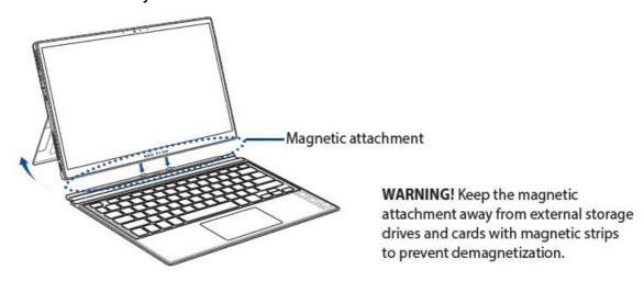
**WARNING!** Keep the magnetic attachment away from external storage drives and cards with magnetic stripsto prevent demagnetization.
