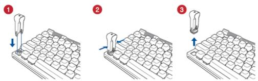
**CAUTION!** Be careful when removing or replacing the switch; damages to the switch and/or the keyboard due to removing or replacing the switch is not covered by the warranty.
