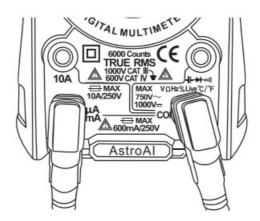
• Under the A setting, connect the red test lead to the 10A terminal and the black test lead to the COM terminal.
