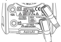
• Turn the rotary dial to the v set. When the voltage is below 600mV, turn the dial to the mv setting. Press the "FUNC" button to switch between AC/DC voltage. The screen will indicate the setting that the DMM is currently in. "DC" will display for DC measurements and "AC" will display when the Meter is set to measure AC.
