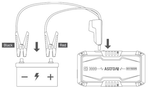
2. Operate the jump starter according to the indicator on the smart battery clamps.
