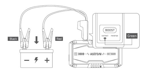
• When the smart battery clamps' indicator is illuminated green, jumpstart your car.
