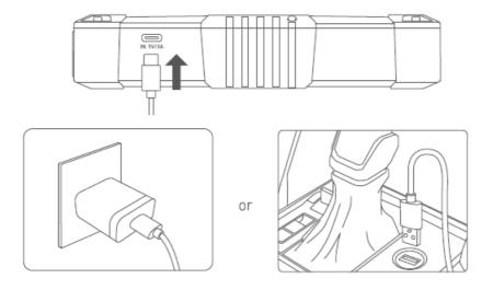
**Note:** The battery indicators will illuminate circularly while charging; the illuminated indicators represent the current battery level. If all four of the battery indicators are off, it means the charging is complete.
