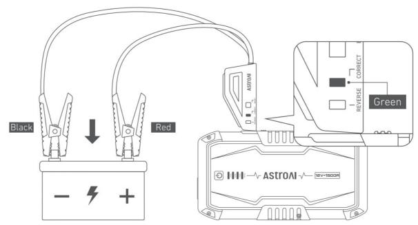
3. When the smart battery clamps' indicator is illuminated green, jumpstart your car.
