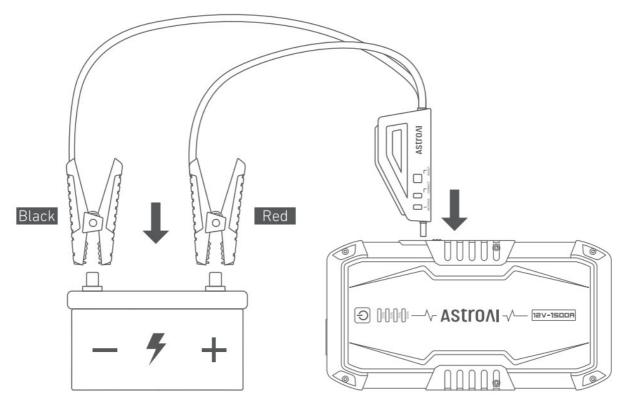
2. Operate the jump starter according to the indicator on the smart battery clamps
