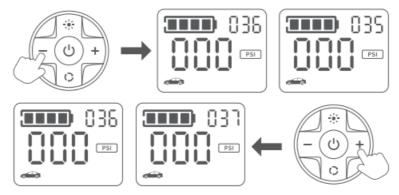
3. Press the Power Button to start inflating. The machine will automatically stop when the inflation is complete. Tip 1: To avoid overinflation, please confirm the maximum inflation pressure of the objects being inflated. Overinflating may cause explosions and personal injuries.
