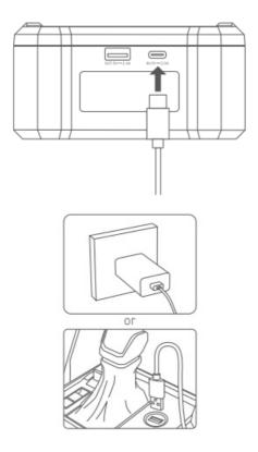
While charging, the power bars will flash from one to another. When a bar changes from flashing to fully illuminated, it is charged to that level. The remaining bars will continue flashing in a cycle until all four bars are illuminated. The screen will turn off when the charging is complete.
