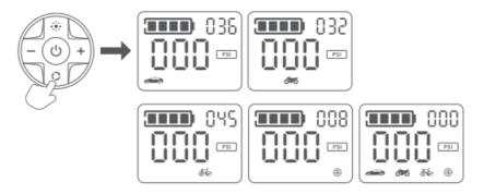
2. Press and hold the Mode Button to switch units between Bar, PSI, and kPa
