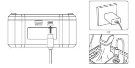
While charging, the power bars will flash from one to another. When a bar changes from flashing to fully illuminated, it is charged to that level. The remaining bars will continue flashing in a cycle until all four bars are illuminated. The screen will turn off when the charging is complete.
