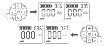
3. Press the Power Button to start inflating. The machine will automatically stop when the inflation is complete.
