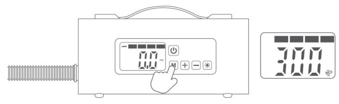
Press the "+" & "-" buttons to adjust inflation/deflation time. The default time is 300 seconds.
