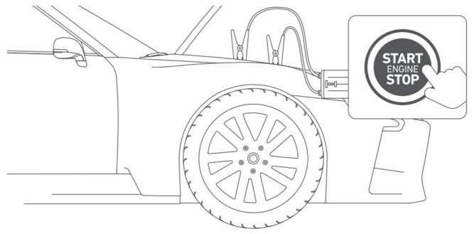
4. Remove the smart battery clamps from the battery.
