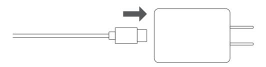
2. Connect the USB-C end of the USB charging cable to the Type-C port of the product.
