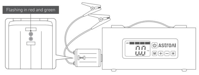
2. Connect the smart battery clamps to the vehicle's battery. Iluminated red, buzzer long beeping Cause: Short circuit Solution: Check the circuitor ry step 1 Iluminated red, buzzer emitting a short beep sound Cause: Reversed polarities Solution: Reverse the clamps.
