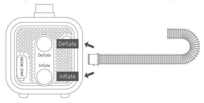
2. Choose a nozzle based on the items being inflated or deflated, horizon- tally align the hose and accessory nozzle, twist them clockwise along the threads.
