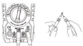
• Turn the rotary dial to the "Ω + " setting. Press the FUNC button to switch to the capacitance test. The screen will display "F" indicating that the measurement function is capacitance.
