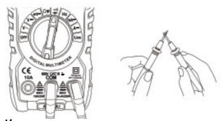
• Turn the rotary dial to the "Ω † " setting. The screen will display "Ω" indicating that the measurement function is resistance.
