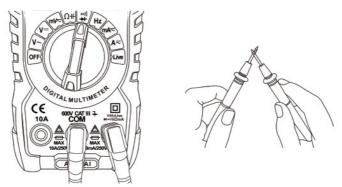
Turn the rotary dial to the "Hz" setting. The screen will display "Hz" indicating that the measurement function is frequency.
