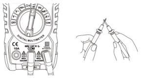
• Turn the rotary dial to the "Live" setting. The screen will display "Live" indicating that the measurement function is a live wire.
