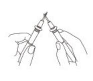
• Connect the test leads to both ends of the circuit or resistance under test (parallel). If the resistance of the circuit or resistance under test is connected and less than 50Ω, the buzzer will emit a beep and the measured resistance value will be displayed on the LCD display.
