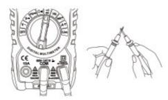
Turn the rotary dial to the "V ~" setting. The screen will display indicating that the measurement function is AC~ voltage.
