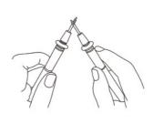
Insert the black test lead into the "COM" terminal and the red test lead into the 10A terminal.
