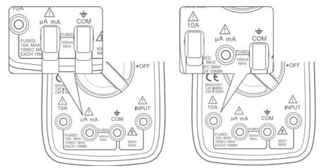
2. Choose functions: Turn the rotary switch to the "µA", "mA' or "A' setting according to the estimated value.
