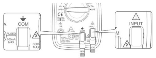
2. Choase functions: Turn the rotary switch to the "Hz/Duty" setting. Press the "Hz/Duty" Button to switch frequency measurement or duty ratio measurement
