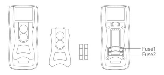
Replace the damaged fuse with a new one with the same ratings. This meter uses two fuses:
