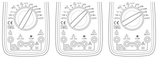
3. Choose current types: Press the "Select" Button to choose between a DC or AC current test.
