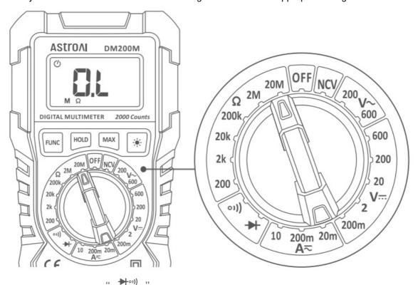
2. Insert the red test lead into the VΩmA terminal and the black test lead into the ""COM" terminal.
