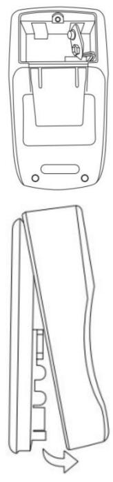
Remove the blown fuses and replace them with new fuses of the same specification, make sure that the fuses are loaded into the fuse clip and clamped tightly.
