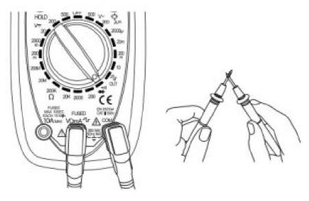
• Turn the rotary dial to the "A=" area with yellow font. The screen will display "000" indicating that the measurement function is a DC A current from 200pA to 200mA.
