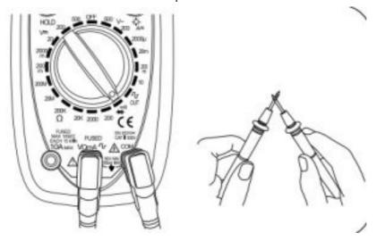
• Turn the rotary dial to the "" setting. The screen will display "1" indicating that the measurement function is square wave output.
