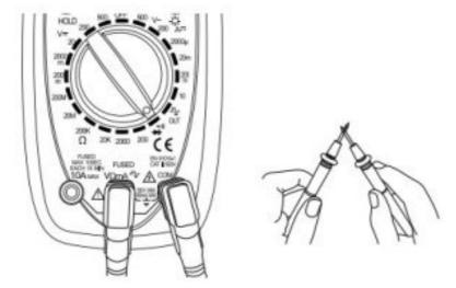
• Turn the rotary dial to the "CI" area with a yellow font. The screen will display "1" indicating that the measurement function is resistance.
