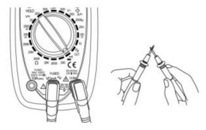
Insert the black test lead into the "COM" terminal and red test lead into the 10A terminal.
