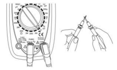
• Turn the rotary dial to the "V-" area with a white font. The screen will display "000" indicating that the measurement function is DC voltage.
