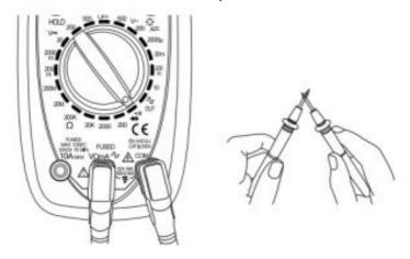
• Turn the rotary dial to the "V" area with a white font. The screen will display "000" indicating that the measurement function is DC voltage.
