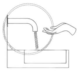
When the hands are removed a decrease is detected, turning off the water and returning the tap to standby mode.
