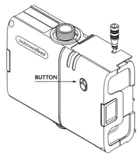
After adjusting the level, press the button for 5 seconds to validate. The 2 green and red LEDs will flash once. After adjustment, the system will reboot and restart 1 cycle of auto-calibration (STEP 10)
