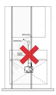
**NOTE**: The plumbing fittings including sensor box in-wall must not be within 250mm of conductive materials including steel framework, mirrors and other copper plumbing.
