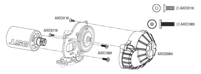
Remove the transmission cover and output gear assembly.
