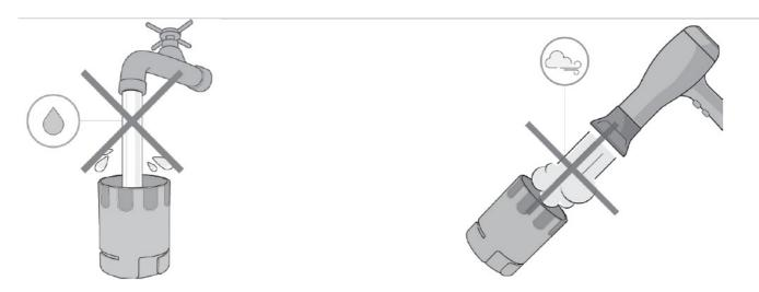
Correct operation of the turbine is guaranteed only if it is "clean" and free of foreign objects that affect its movement. The presence of dust or foreign bodies (such as hairs, sputum etc.) could slow or block the moving parts of the turbine and make the result less accurate, or damage the turbine itself.
