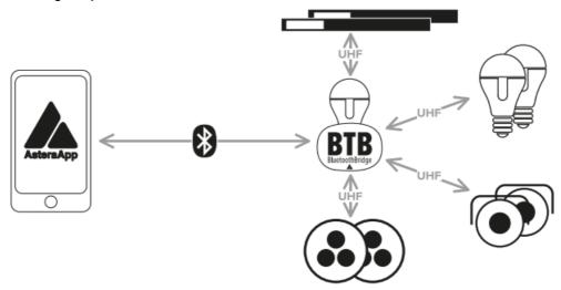
Please power on the light. Hold down the power button for 3 seconds until the light flashes blue. In the AsteraApp press "Manage Bluetooth Bridges", then "+" and follow instructions on screen to connect. The light which is connected as BTB shows a small Bluetooth Icon in the display.
