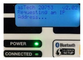
3. Then the CONNECTED lamp will illuminate and the screen will display Connected & Waiting. Your asTech device is now connected to our remote servers. After you submit your Service Request, one of our Technicians will pair your vehicle with the appropriate OEM tool to perform the requested work.
