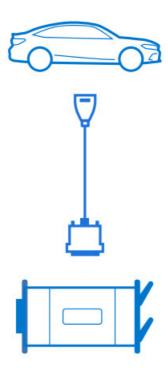
Plug your asTech Device into a vehicle place the ignition in On/Run, engine off. An IP Address, VIN, and "Connected & Waiting" should appear on the device screen. The device is now ready to use.
