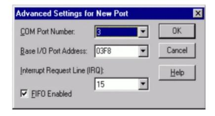
To add a COM port, use START|CONTROL PANEL|PORTS applet and click ADD, then enter the correct UART address and Interrupt number. When the "Add New Port" dialog is configured click OK, but answer "Don't Restart Now" when prompted, until you've added any other ports as well. Then restart the system normally, or by selecting "Restart Now."
