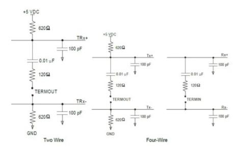
Figure 3-2: Simplified Schematic – Two-Wire and Four-Wire Connection
