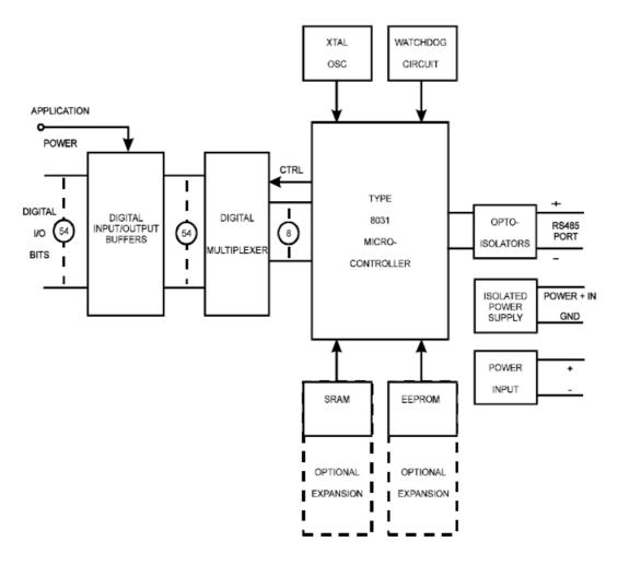
The built-in watchdog timer resets the pod if, for some unexpected reason, the microcontroller "hangs up". Data collected by the pod can be stored in local RAM and accessed later through the computer's serial port. This facilitates a stand-alone pod mode of operation.
