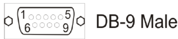
Figure 6-1: Male DB9 Connector Pin Locations
