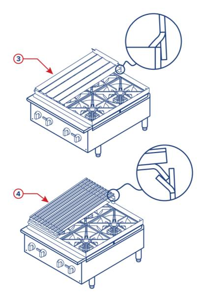
**STEP 4.**Rotate drip tray under front lip of griddle/broiler.
