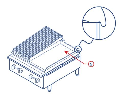
Set the broiler onto frame using the 2 hooks in the rear. Set broiler grates onto the broiler using the 2 hooks in the rear.
