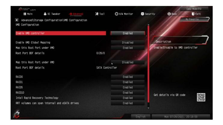
Then set Enable VMD Global Mapping to [Enabled]. Next, press < F10 > to save the configuration changes and exit setup.
