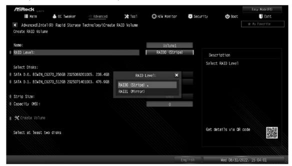
• STEP 7: Select the hard drives to be included in the RAID array and press <Enter>.
