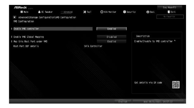
Then set Enable VMD Global Mapping to [Enabled]. Next, press <F10> to save the configuration changes and exit the setup.
