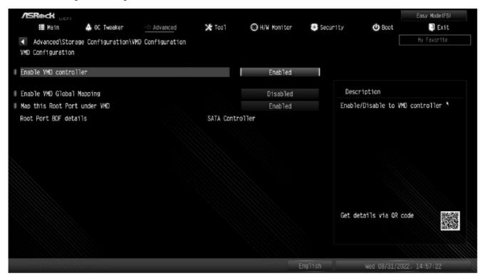
Then set Enable VMD Global Mapping to [Enabled]. Next, press <F10> to save the configuration changes and exit setup.
