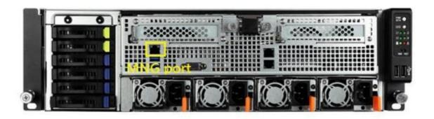
b.) For some ASRR Server Systems which support to NCSI function, you can also connect your System to Local Area Network via either System's MNG or LAN1(shared IPMI LAN) port:
