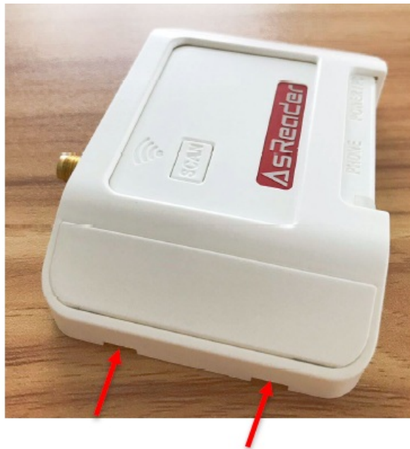
FIG. 5-6 Method of removing the lids
