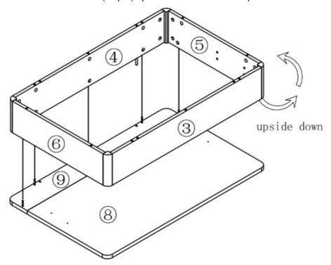
STEP #9 Put 5 cam bolt nuts (part B) inside the holes on panel 4&5&6, then screw to lock them.
