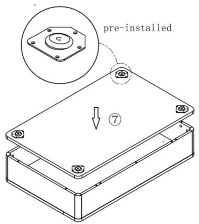
STEP# 14 Fasten 4 solid wood legs on to pre-assembled metal plates on panel 7
