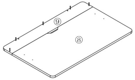
STEP #8 Tum the assembled table frame (step 5) upside down then Fit it on panel 8 & 9.
