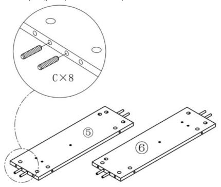
STEP #3 Insert 2 wood dowel pins into each side of panel 3 & 4, and 2 wood dowel pins into top of panel 4.
