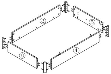
STEP #5 Put 16 cam bolt nuts (part B) inside the holes on panel 3-6, then screw to lock them.
