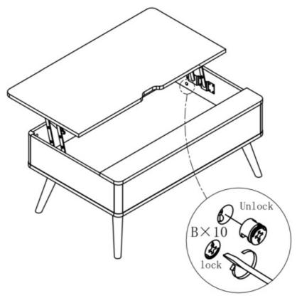
STEP #17 Place metal bar (Part I 0) between two lift mechanisms, fasten two m6 screws (part F) into it.
