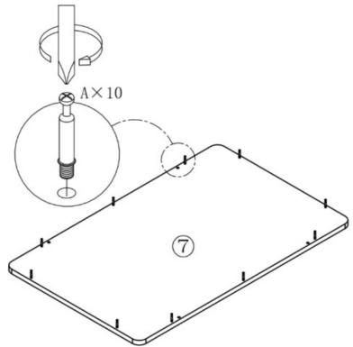
STEP# 13 Fit panel 7 onto table frame, align the bolts and pins carefully.
