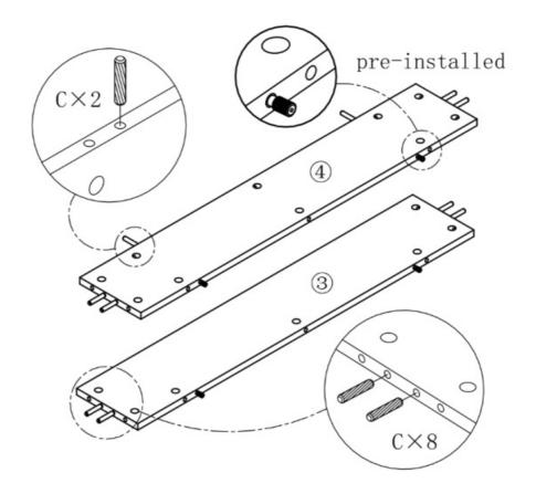
STEP #4 Put rounded bars (part 2) and panel 3-6 together.
