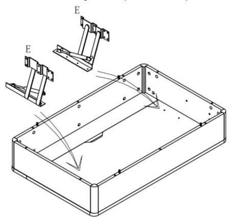
STEP # 11 Find IO m5 screws and fasten lift mechanisms to the panel 5 &6& 8.
