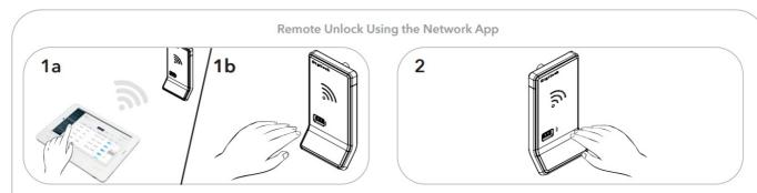
**Unlock**: Locate the specific lock that you wish to remotely unlock on the hardware list within the Network app. Toggle the switch next to the lock name to unlocked. Present hand to the lock interface to unlock.
