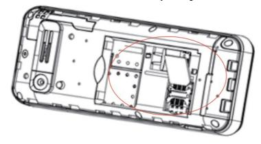
6. With the metallic contacts of the battery facing the metallic contacts in the battery slot, press the battery down until it locks into place. You can then re-install the back cover.
