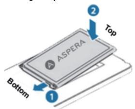
4. Pull the battery up from the top left and then lift the battery away.
