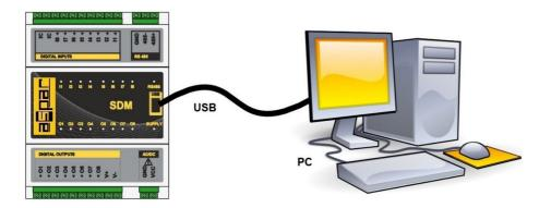
Modbus Configurator is software that is designed to set the module registers responsible for communication over Modbus network as well as to read and write the current value of other registers of the module. This program can be a convenient way to test the system as well as to observe real-time changes in the registers.
