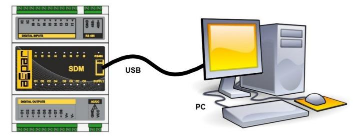
Communication with the module is done via the USB cable. The module does not require any drivers. Configurator is a universal program, whereby it is possible to configure all available modules.
