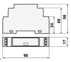
Look and dimensions of the module are shown below. The module is mounted directly to the rail in the DIN industry standard.
