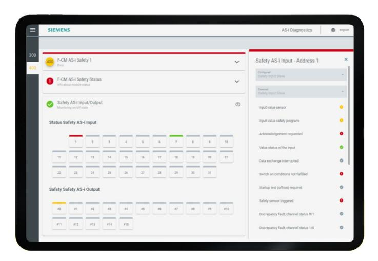
By touching or clicking on the block icon of a safe input/output, further diagnostics data for fault determination is displayed on the right side of the screen.
