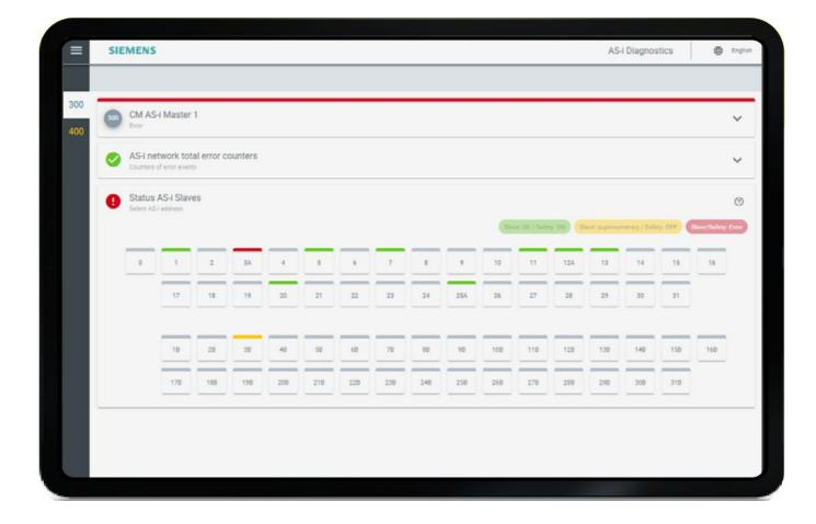
Benefit for the user: He or she logs on to the CPU only once and can call up the diagnostics for all connected AS-i networks. And for the administration, this means that only the port of the CPU web server has to be secured against unauthorized access, but not every single AS-i master gateway.
