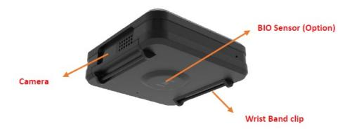
**BIO Sensor (Option):** The function of BIO sensor is to detect the heart rate. It should be touched well with wrist when wearing with the wrist band.
