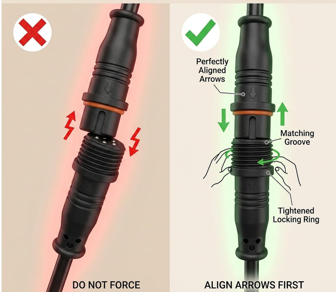
Figure 3: Important note on connecting pump components. Align arrows first to prevent damage.
