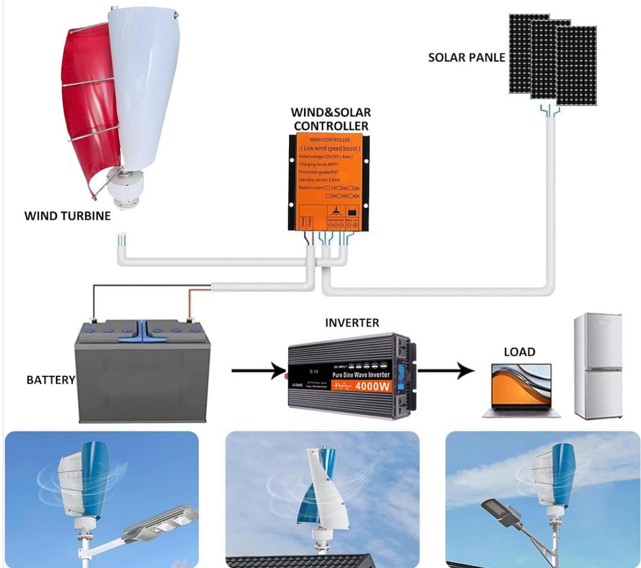
Image 5.1: Diagram illustrating the connection of the wind turbine, solar panels, controller, battery, and inverter in an off-grid hybrid system.
