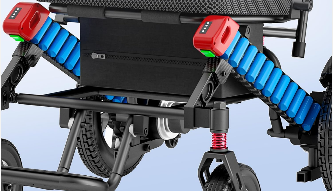
Image 6.2: The dual battery compartment design, illustrating the range provided by single (12 miles) and dual (24 miles) batteries.
