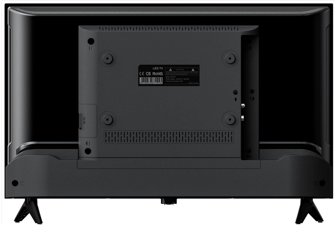
Image: Rear view of the TV, illustrating the VESA mounting points and the areas where the stand legs attach.
