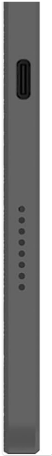
Image: Close-up of the POGO PIN connector, used for attaching the keyboard.
