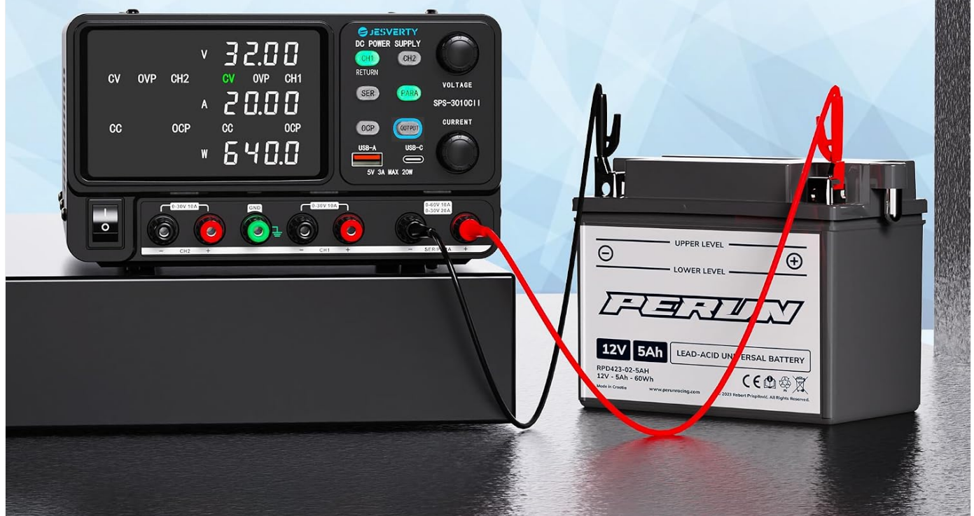
Figure 5.5: Illustration of the power supply connected for battery charging, showing compatibility with various battery types.
