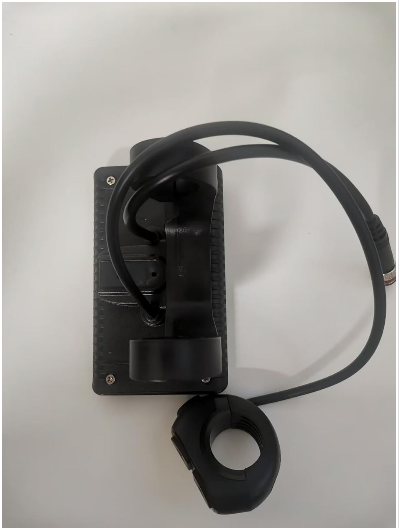
Figure 2: Rear view of the King-Meter SW-LCD display, illustrating the integrated mounting bracket and the attached cable for connection to the e-bike system.
